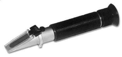
This Salinity Refractometer is for quick and easy measurement of the salinity in water. This simple to use refractometer measures in parts per thousand (ppt) or specific gravity. The meter operates with natural light and has no moving parts to wear out. Hatchery and farm tested for reliability and durability.
