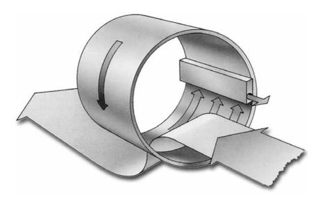
Microsieving is an efficient and reliable technique for separation of particles from all kinds of liquids. Hydrotech develops and manufactures high performance filters for water purification and product recovery.
