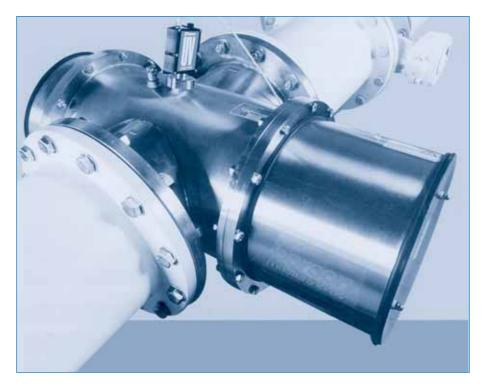
An alarm is given when the UV-dose drops below a preset level. This for example can be caused by extra pollution of the incoming water. The guartz tubes in the UV-chamber can be cleaned with a manual or automatic wiper, even when the unit is in function.
