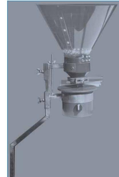
CJ offers a range of highly reliable feeders with a wide field of applications. Due to its uniform construction the motor unit and pendulum are exchangeable, enabling the farmer to use the feeder for early weaning with motor or apply appetite feeding using the pendulum.
